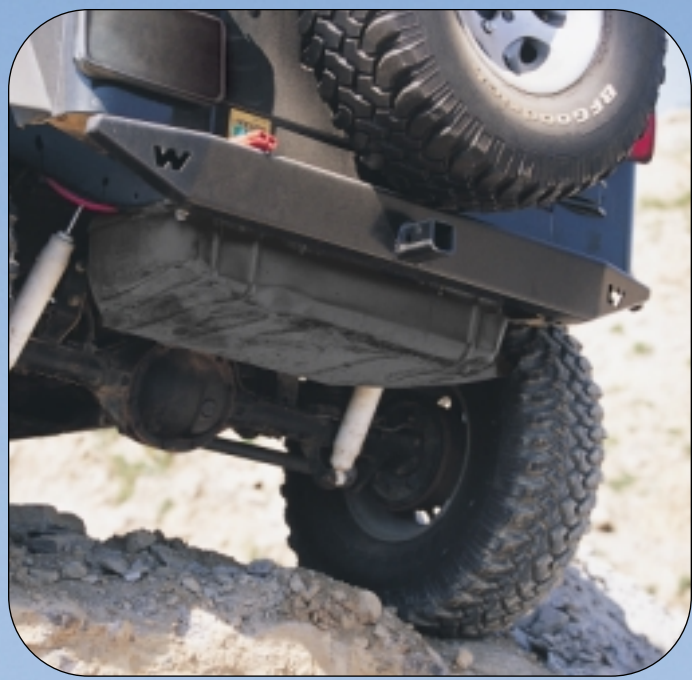
Rear bumpers have a 2" receiver for using the Warn shackle bracket (PN29312) to increase your recovery options.
