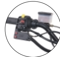
Handlebar switch allows the rider to operate the actuator without removing the hand from grip
